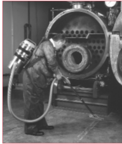
The Compact Vac with wheeled floor nozzle for general cleanup.
